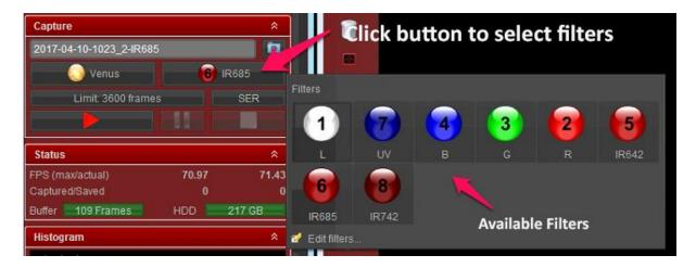
To select filters simply click the filter button indicated to bring up the selection available. Again note Firecapture will automatically refocus for each filter one you have calibrated the focus positions.
