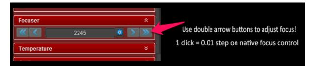
Focus control can be seen in the Firecapture sidebar. Use the DOUBLE ARROWS to make focus adjustments as this corresponds to the smallest step on the native focus control.
